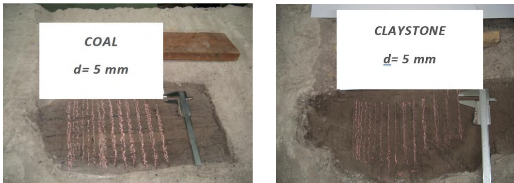
Figure 3. Cutting tests samples were performed for 5 mm depth.
