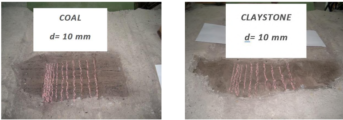
Figure 4. Cutting tests samples were performed for 10 mm depth.
